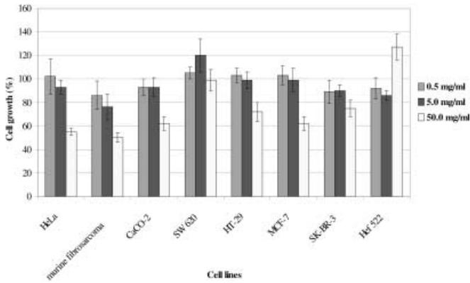
**Fig. 2** Effect of the medium pretreated with 0.5, 5.0, and 50.0 mg/ml MZ on growth of various cell lines. Vertical bars Standard deviations; all white bars (50 mg/ml) are statistically different in comparison to control ( $P < 0.001$ , Student's *t* test)
